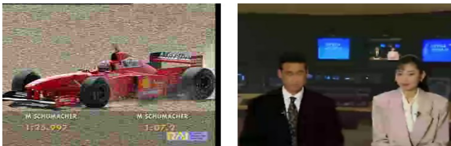
Figure 1: video degradation with blockiness (left) and blurriness (right) (from [5])
